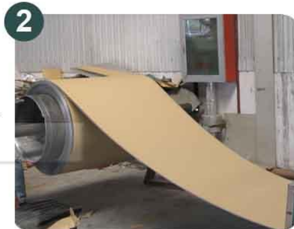
2. In Strict Accordance with ASTM C1729, the moisture retarder has no visual defects that will affect the performance. And it's free of laminated separations, holes, rips, tears, scratches or dents.
